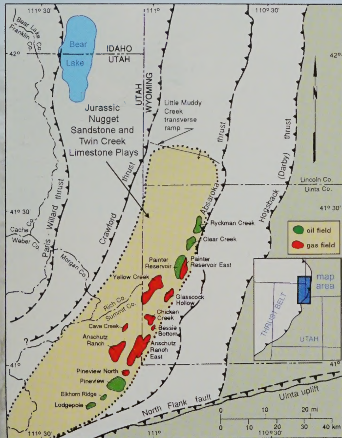
Oil and gas fields, uplifts, and major thrust faults (sawteeth) in the Utah-Wyoming thrust belt. Future exploration could focus on more structurally complex and subtle, thrust-related traps using 3-D seismic surveys with any new fields developed by horizontal drilling.
